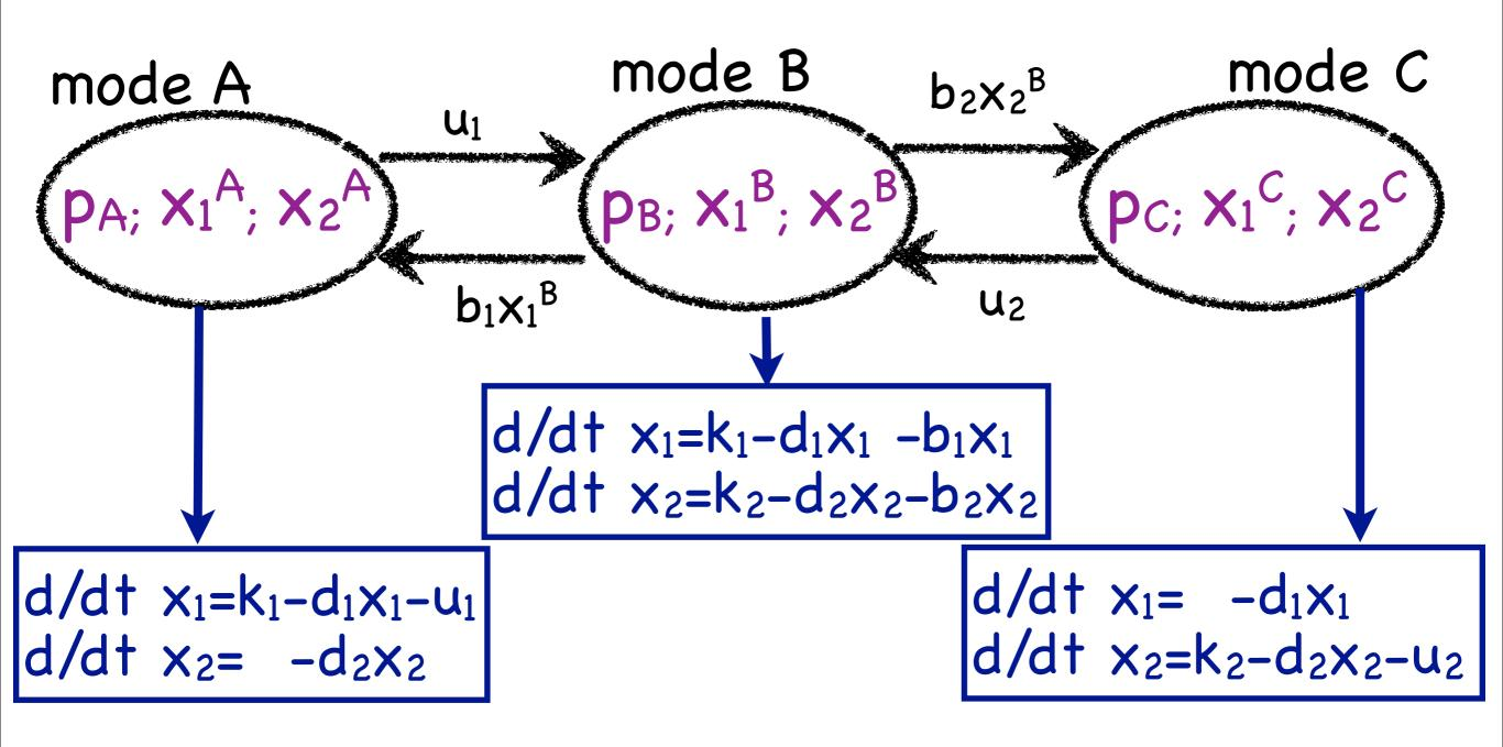
Result at t+h: new probabilities  $p_A(t+h), p_B(t+h), ...$ and new conditional expect.  $x_i^A(t+h), x_i^B(t+h), ...$
