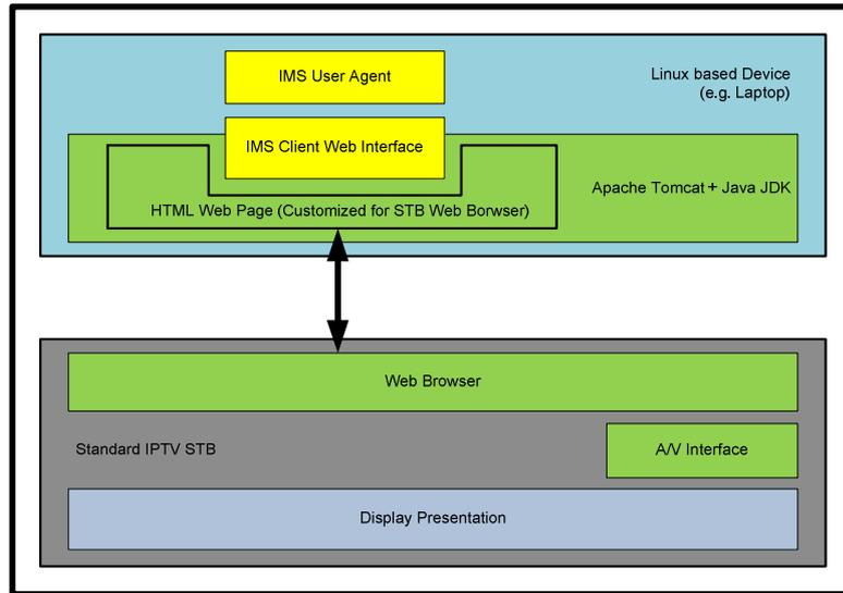
**Figure 4 Architecture of the Mobicome IMS-IPTV client prototype**
