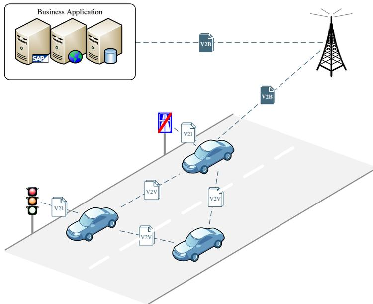
**Fig. 1.** State-of-the-art communication technologies enable vehicles to communicate among each other (V2V), with their surrounding roadside infrastructure (V2I), as well as with with business applications of services providers (V2B)
