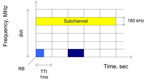
**Fig. 1.** Radio resource structure in LTE networks.
