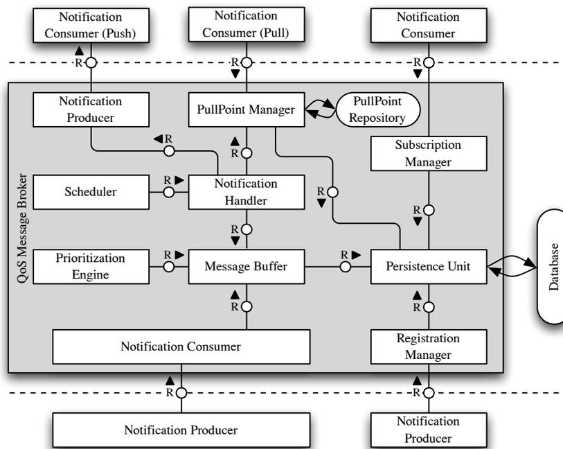
**Fig. 2.** Overall design of the in-vehicle QoS message broker
