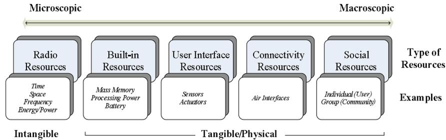
**Fig. 1.** A classification of resources in wireless networks.
