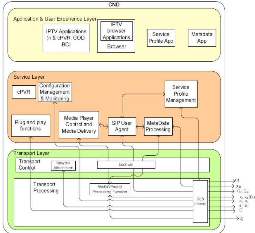
**Figure 1 The architecture of the TISPAN IPTV CND**
