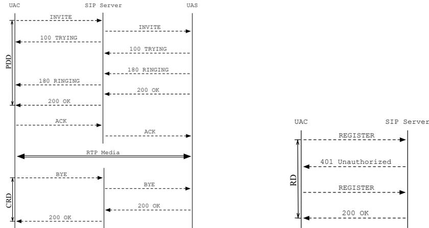
(a) Message flow for call setup and tear-down.
