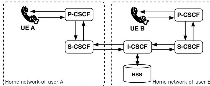
Fig. 1. Call routing between networks.
